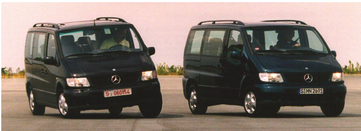
Fig. 11: Model-based comfort control in V class with hydropneumatic suspension struts. Comparison between passive (left) and active (right) while cornering
