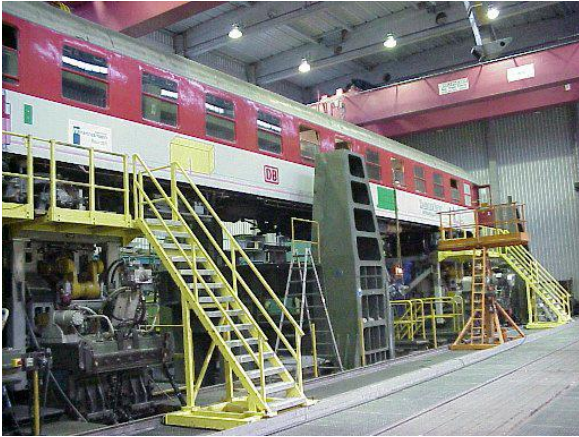
Fig. 10: Model-based lateral comfort control for high-speed trains on a dynamometer in Munich
